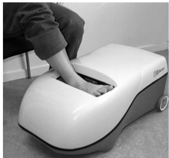
Figure 1 The DXL Calscan device used in the osteoporosis management system. The measurement time is 55 s and the absorbed dose to the patient less than 0.2 \mu Sv.
